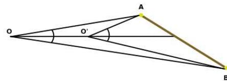
Fig. 3. The sensitivity of the angle increases as the vessel draws closer to the range lights.
