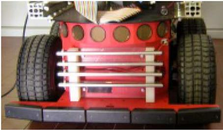
Fig. 5. Photograph of the electrical bar contacts mounted onto the robot.
