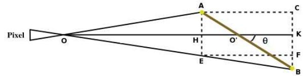
Fig. 7. The accuracy in alignment of our vision system: though points A and B are believed as in line, the real dimensions of the pixel cause an error ( $\theta$ ) of positioning.
