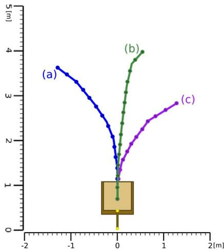
Fig. 13. Odometry traces measured during three docking tests.
