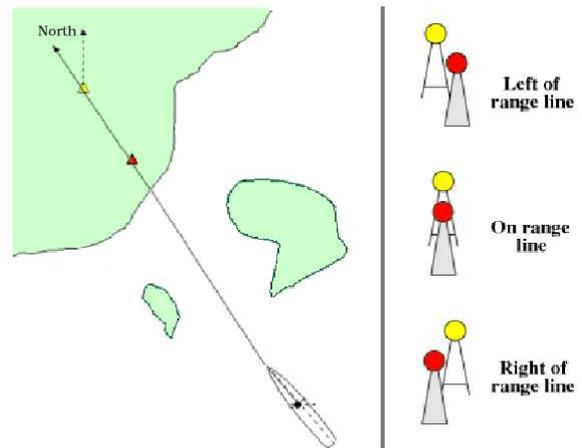
Fig. 1. Range lights are widely used in sailing, to indicate a safe route passing through channels or entering ports, avoiding dangerous obstacles.
