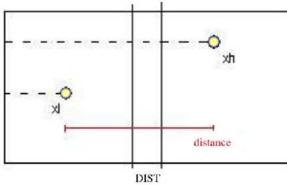
Fig. 10. *Distance* supply the direction of the robot regarding the station. The robot comes from the right so the value of *distance* is positive.
