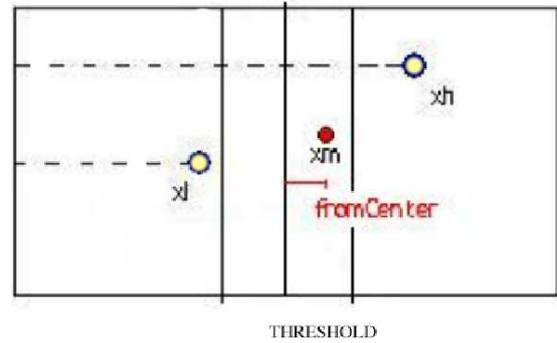
Fig. 12. *fromCenter* is lower than *THRESHOLD*, so the robot is on the axis of the docking station.
