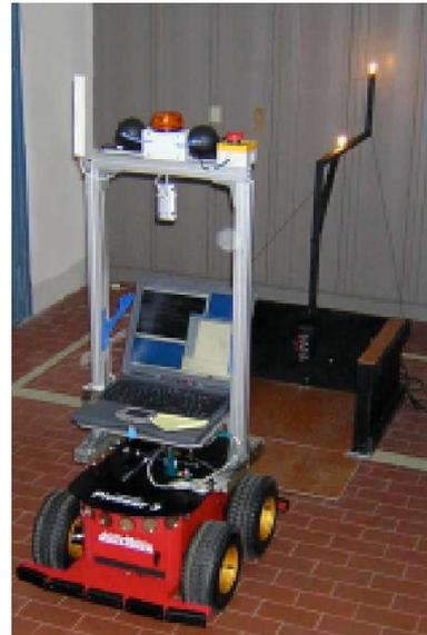
Fig. 2. The whole system: photograph of the robot docking into the charging station.
